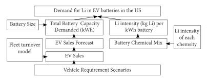
Figure 9. Modeling approach for estimating lithium demand from EVs in the US
