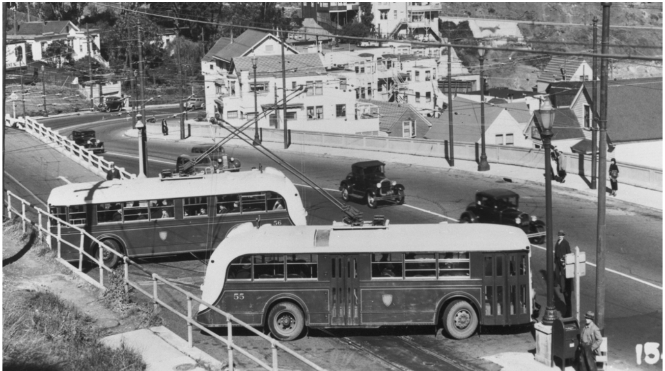
JG Brill Trolley Coach, Two of the first Electric Rubber Tire Transit Vehicles in San Francisco. 1935. Muni Photo Archive.
